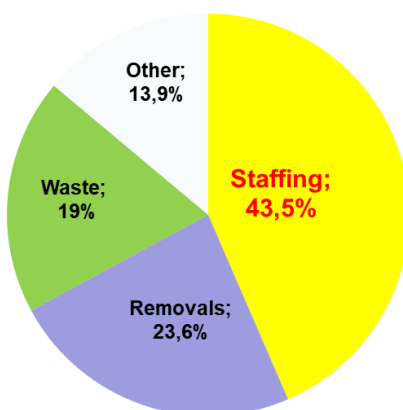
Figure 14-1: Example of breakdown of decommissioning costs for a PWR/BWR in the US [49].
